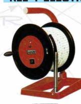
The SEBA-KLL-T has been developed for accurate measurements of water level ande temperature in groundwater observation tubes and wells.
