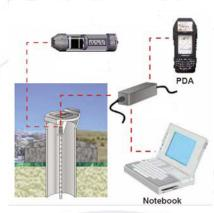
System for measuring groundwater level
