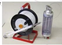
The liquid sampler KLL-S is designed for operation inconnection to the approved SEBA Electric Contact Meter.In this combination liquid samples can be taken in any desired depth.
