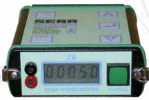
With this full-electronic counter it is possible to receive frequencies for all flow velocities. The impulses generated by the current meter are added and indicated in relation to the preselected time. The timing startsfrom the first impulse.
