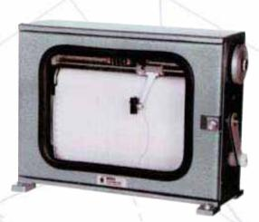
The strip chart water level recorder DELTA serves for continuous registration of water leveks in flowing and stagnant waters. The registration will be effected on a 16m long diagram roll. Mainly this instrument will be used for r :
